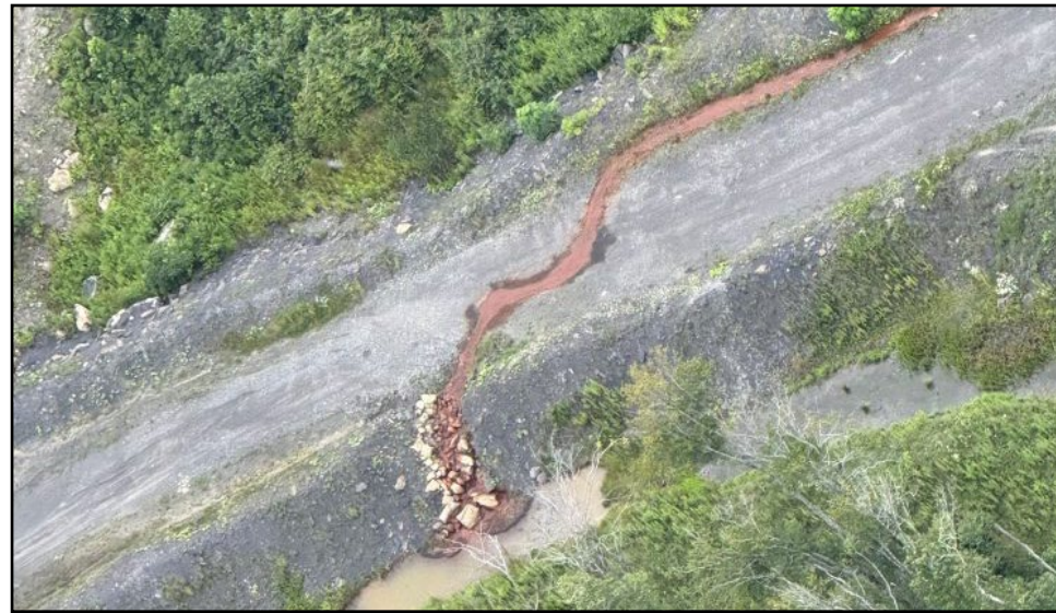
Orange water, indicative of acidity and high levels of iron, discharging from South Fork Coal’s Lost Flats mine, flowing towards the South Fork of Cherry River.
